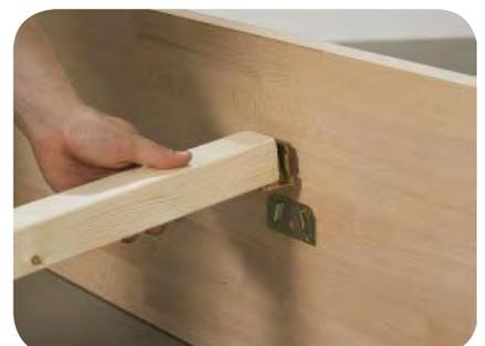
4. Pre-drill holes for supporting timbers. Countersink holes pointed towards centre of bed. Mount supports with screws (4x60).
