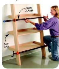
7. Lift the ladder shelf and place it upright against a straight wall. Check it with a framing square and flex it if necessary to square it up and to make sure that the uprights rest flat against the floor and wall (assuming your floor is level). Attach three bar clamps while the glue dries.
