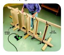
6. Carefully turn unit over and repeat the process to attach the second upright. Work quickly so the glue doesn't set.
